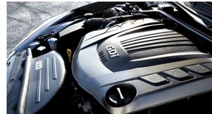
**AN INJECTION OF POWER** With every rev of its 348-horsepower GDI V6, fuel is injected directly into the cylinder, creating potent-yet-efficient combustion. Genesis Coupe's powerful stopping performance is aided by available 4-piston Brembo® brakes.
