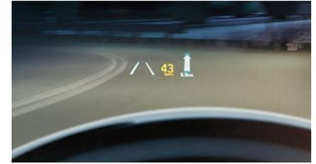
**HEADS-UP DISPLAY** Vital driving information is projected onto the Equus Ultimate windshield for at-a-glance decision making: Driving speed, turn-by-turn navigation, Smart Cruise Control status and alerts for Lane Departure Warning and Blind Spot Detection.
