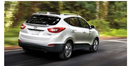
**ALL WHEEL GRIP** To help optimize traction when the going gets tricky, Tucson's available All Wheel Drive continuously varies the torque transfer between the front and rear wheels. Drivers can select the 50/50 torque-split setting to balance power between front and rear wheels in snow or sand.
