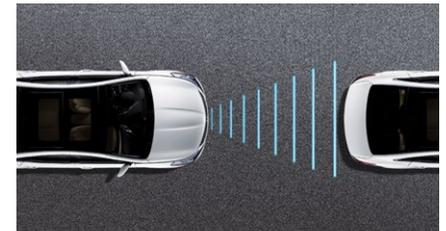
**FORWARD THINKING** Azera Limited comes standard with Forward Collision Warning. A forward-sensing camera looks down the road to determine the closing speed of your vehicle in relation to the vehicle ahead, and provides both audible and visual warnings to alert the driver of a potential collision.<sup>3</sup>
