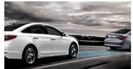
**SMART CRUISE CONTROL** Radar is used to maintain a desired speed and distance from vehicles in front of you. When traffic stops, the stop/start feature brings you to a full stop automatically, then re-engages if the vehicle ahead moves forward within 3 seconds.
