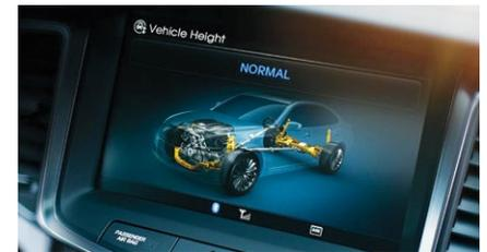
**ELECTRONIC AIR SUSPENSION** The silky smooth Equus ride comes from an Electronic Air Suspension you can set for Normal, Sport and Snow modes. Continuous Damping Control optimizes suspension response during acceleration, braking, cornering and on uneven roads. At higher speeds, ride height lowers for improved stability.
